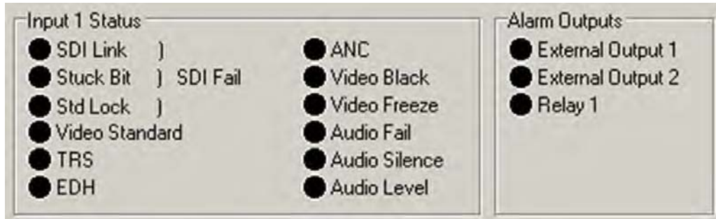
Input 1 status (and output alarms related to input 1)
