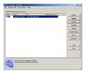
Double click on the *Device Server* icon for the installer to automatically input the settings. The selected IP address should appear. Click *Next* to test the connection to the B064 device server and continue its configuration.
