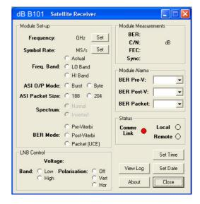
Control is also possible by sending commands to the unit for monitoring and configuration using a standard RS232 terminal or similar application such as Windows® HyperTerminal.
