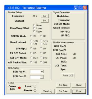
Control is also possible by sending commands to the unit for monitoring and configuration using a standard RS232 terminal or similar application such as Windows® HyperTerminal.
