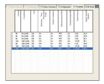
There are 7 pre-programmed DVB-T2 templates which are the UK unified modes. In the UK, Template 7 is the required template.
